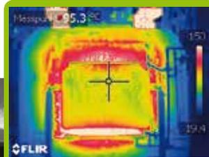
The difference between the insulation of a conventional furnace and ...
