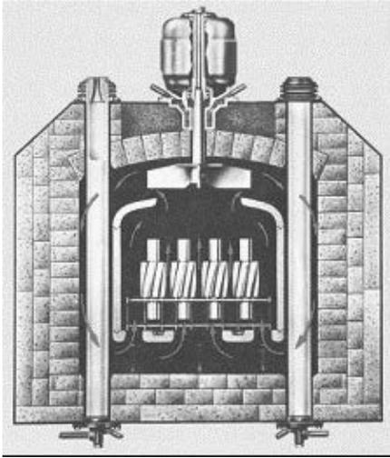
**Fig. 2:** Batch furnaces with muffle
